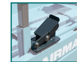
The Slide Deck Extension Release Pedal is capable of unlocking the platform without the user bending.
