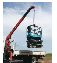
Single point hoisting via the center lifting eye (Option) (Loading image)
